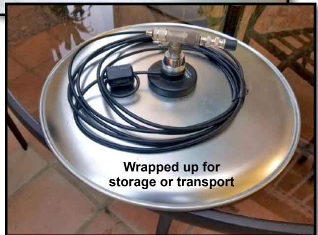
Using a PL-250 "Tee" makes a connector holder and handy handle
