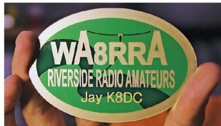
Figure 1 — These WA8RRA club badges were made from printed circuit boards, converted from the club’s logo design. [Jay McClellan, K8DC, photo]
