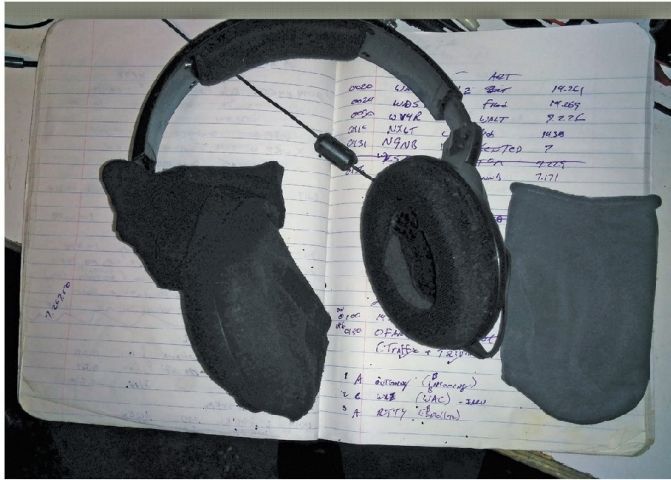
Figure 2 — Nylon socks stretch over headphone earpieces for a cheap, easy cushion repair. [Ralph Phillips, KE5HDF, photo]
