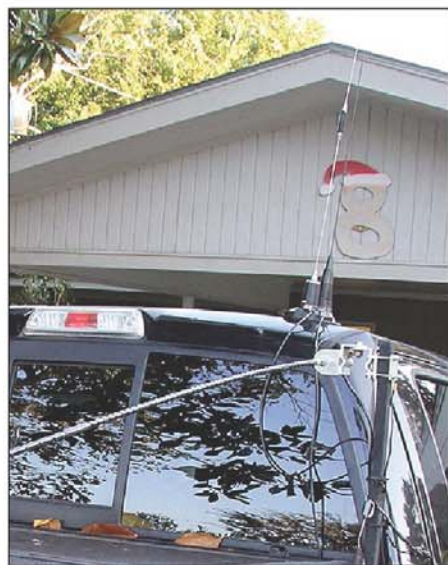
Figure 1 — A quick, inexpensive drop-down mount arrangement that allows you to mount a vertical antenna on your truck. [Mayor Nelson, KD5LBE, photo]
