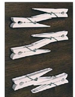
Figure 7 — Clothespins glued back-to-back can be used to support wires in a fan dipole or as clip-on anchors for other applications. [Bob Haynes, WB4AKA, photo]
