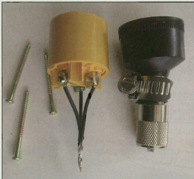
Photo B— How to turn your Christmas lights into an antenna. Just tie together the hot and neutral leads from the lights and wire to the center conductor of the PL-259 coax connector.
