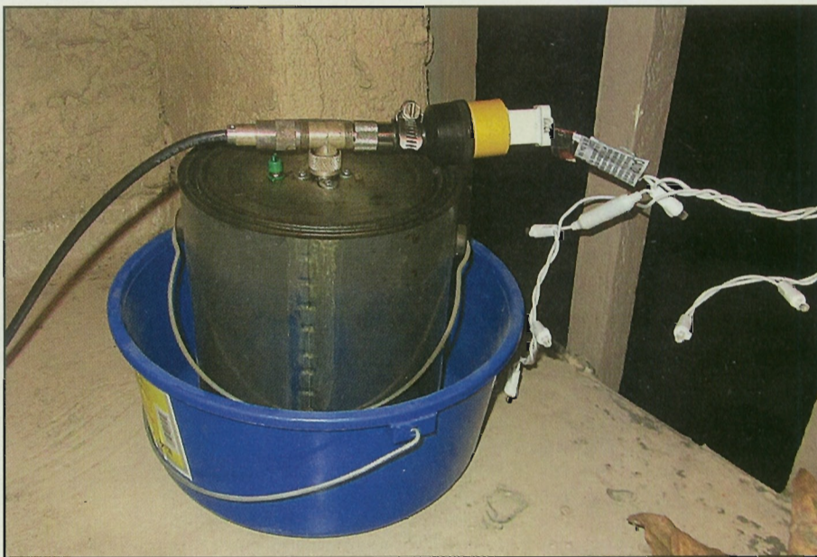
Photo D— The Christmas light adapter connected to the coax tee at the dummy load. Note that the lights are plugged in directly with no additional feedline.
