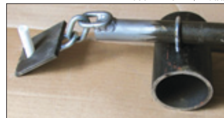
Figure 7 — Joe's removal tool in position and ready to lever the "ground rod" out of the Field Day site.
