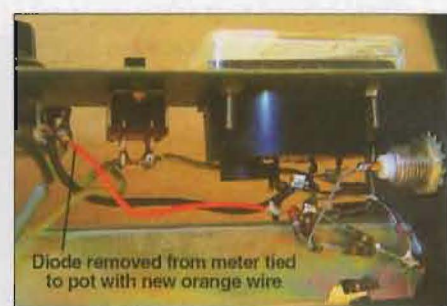
Figure 5 — This wide view inside the SWR meter case shows the new (orange) wire connecting the end of the diode removed from the positive meter terminal with the sensitivity potentiometer.
